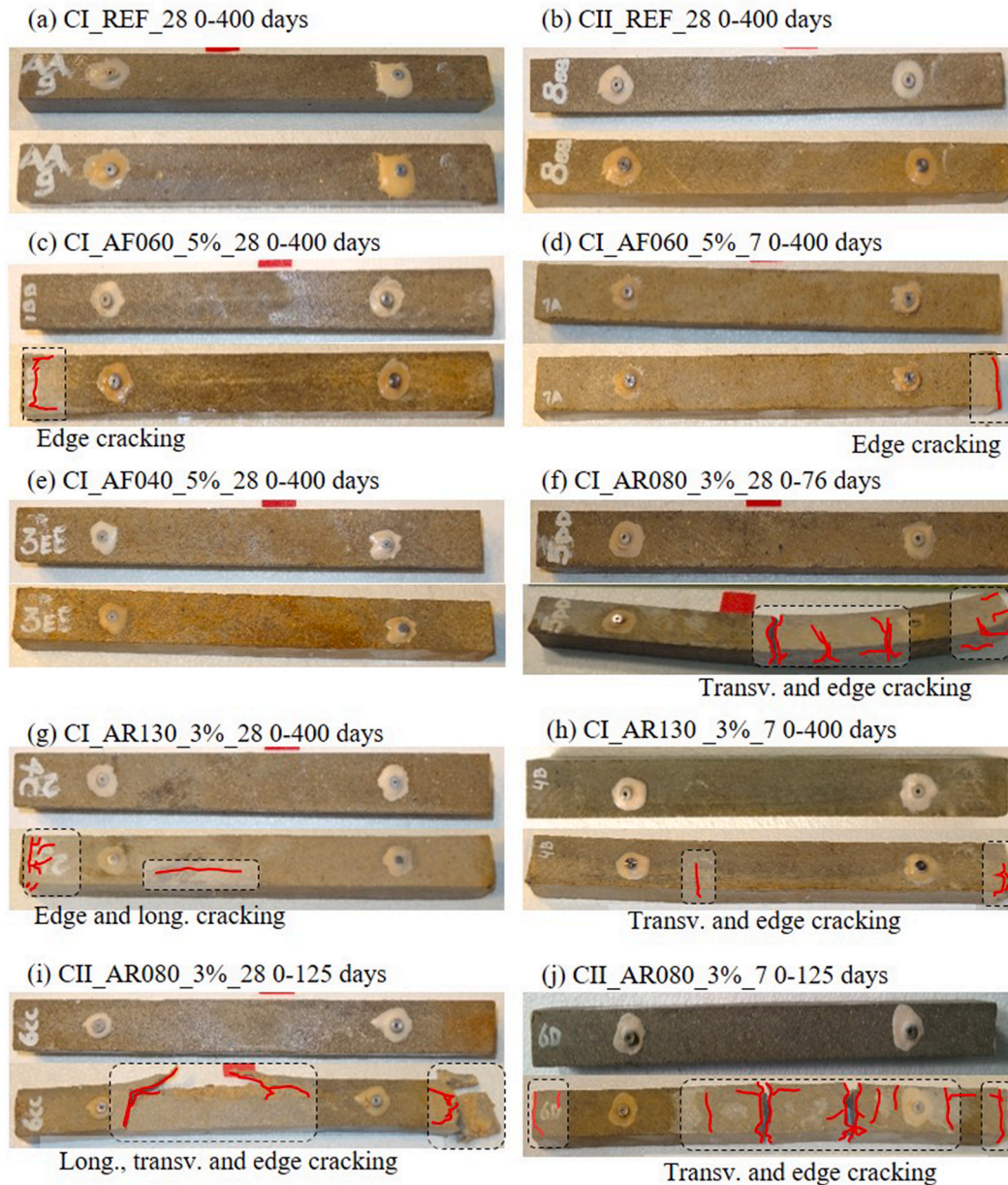
Fig. 4. Visual inspection of the cast and sprayed specimens before and after the accelerated ESA.
