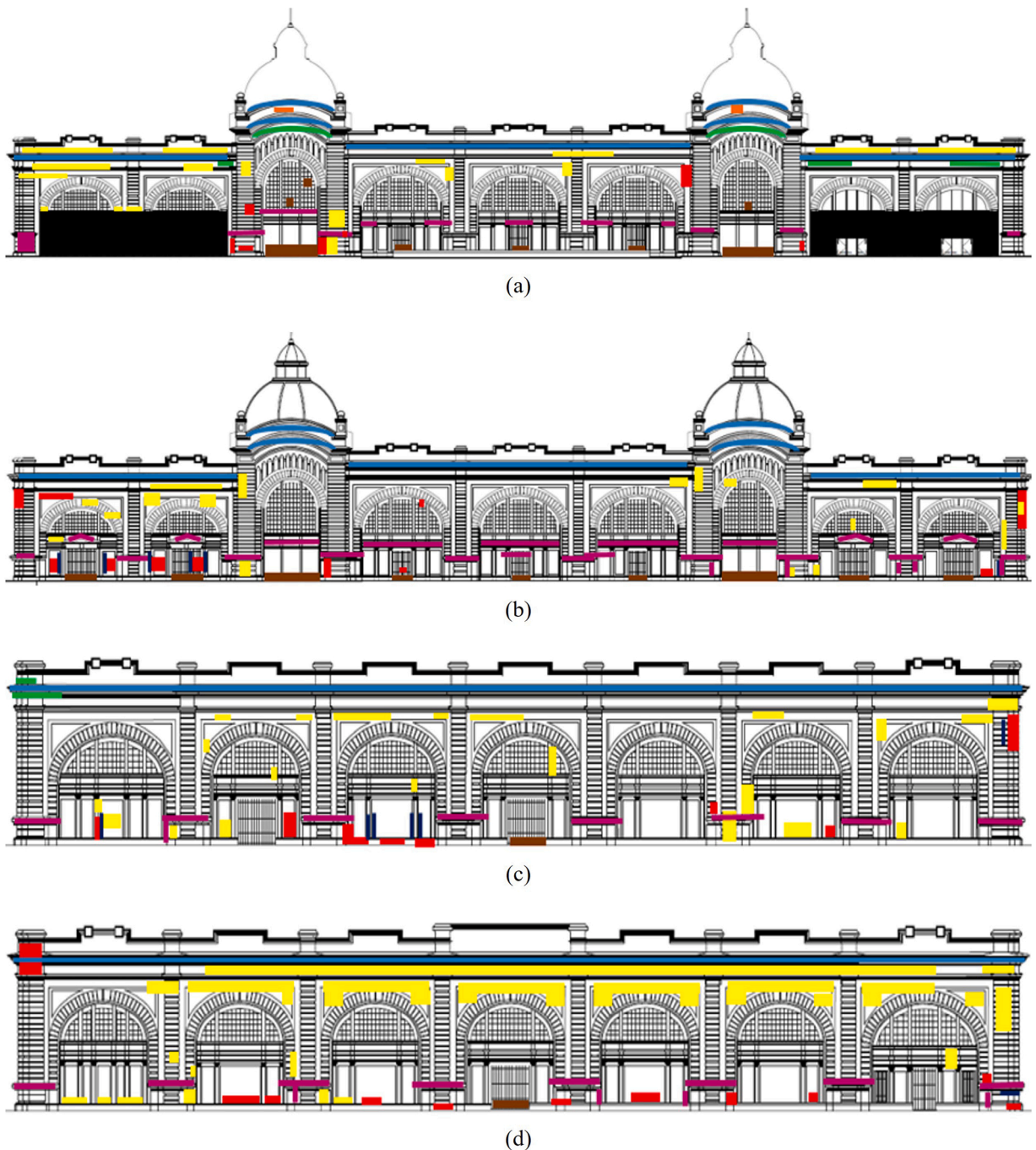
Fig. 7. Mapping of damages on the façades: east (a); west (b); north (c); south (d).
