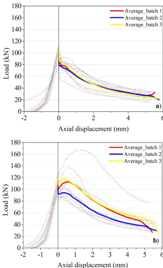
**Fig. 3.** Part 1: load-axial displacement curve from T30(a) and T55(b).
