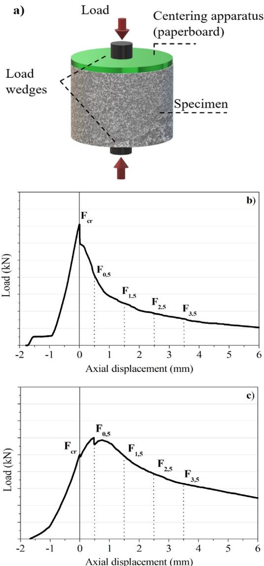
**Fig. 2.** Final set of DPT, with the centering apparatus (a); final load-axial displacement curve with  $F_{cr}$  dislocated to zero value in abscissa axis for softening (b) and hardening (c) behavior.
