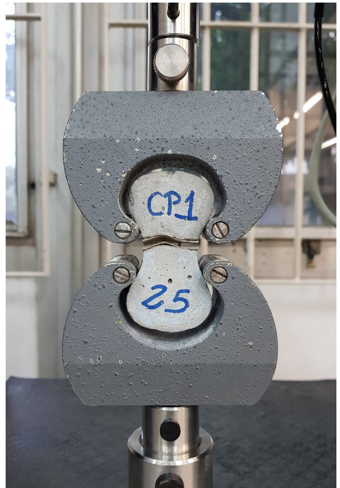
Fig. 7. Pullout test setup conducted in this study.
