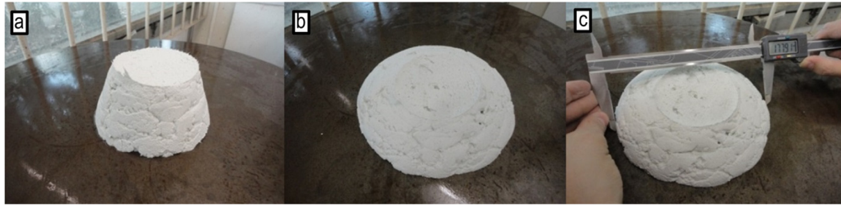
Fig. 5. Consistency according to the flow table method.
