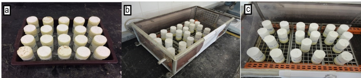
Fig. 10. Water absorption by capillarity. Note – Sample preparation (a); Sub-immersion process (b–c).
