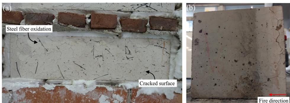
Fig. 6. Physical changes that occurred on the prismatic SFRC specimen after fire exposure.
